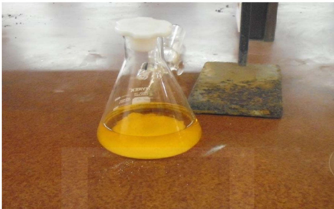
Plate 6b. Drying biodiesel with magnesium sulphate ( \text{MgSO}_4 )
