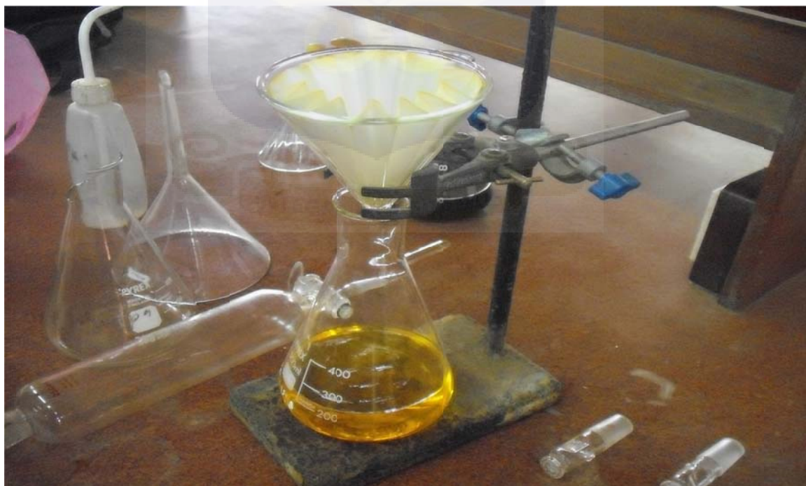
Plate 6c. Separating the drying agent from the biodiesel
