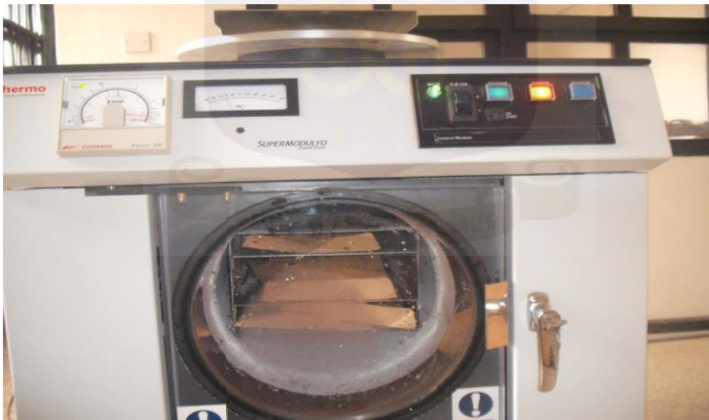
Plate 4. Freeze drying of microalgae in the laboratory
