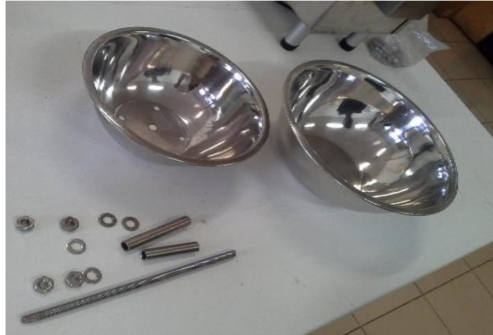
Figure 3-1a: A set of accessories for assembling one passive sampling dome chamber complete
