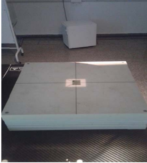
Plate 3.5: RW3 slab phantom with a cut GafChromic EBT3 film placed on it.
