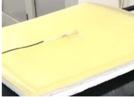
Plate 3.10: Diode taped to Superflab bolus.
