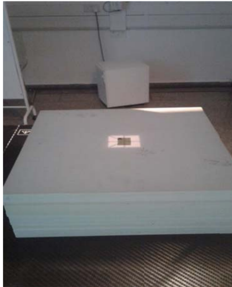
Plate 3.14: Set up for measuring surface dose without bolus using GafChromic EBT3 film.
