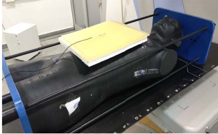
Plate 3.16: Set up for measuring d_{\max} (2.5 cm) dose with 1 cm bolus (15 MV photon beam) using diode and Styrofoam sheets to act as a spacer (air gap).
