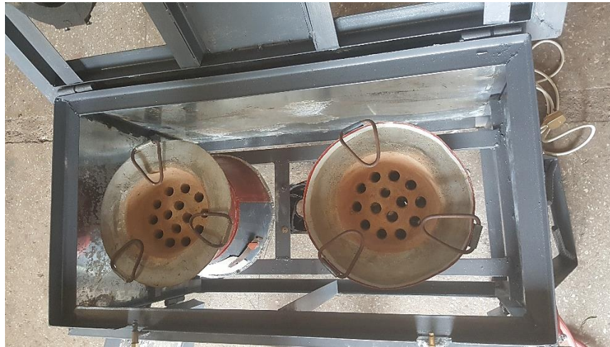
Figure 4.12: View of finished Charcoal compartment of the improved cook stove
