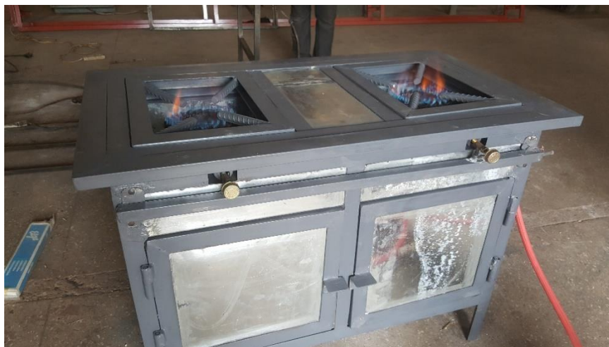
Figure 4.13: View of LPG compartment of the improved cook stove in operation
