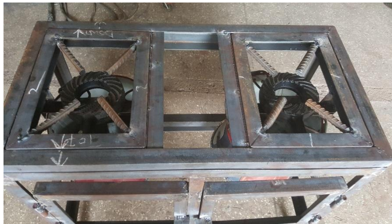
Figure 4.8: The LPG compartment fitted in the upper session
