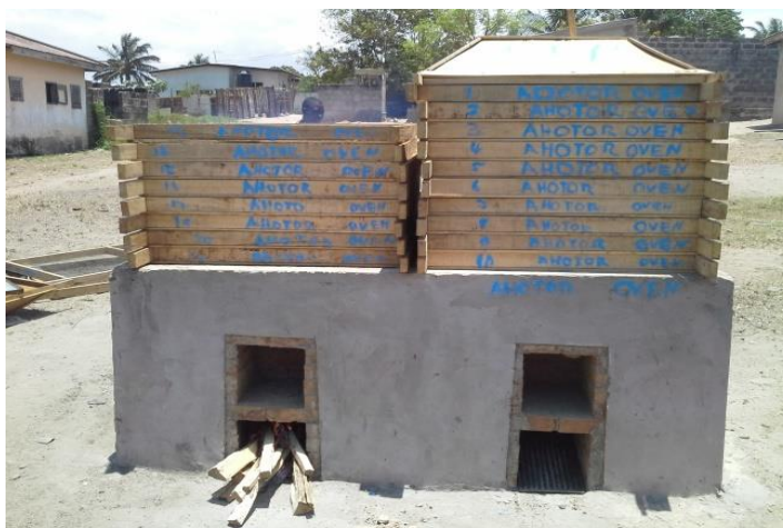
Figure 2.3: Image of the Ahotor Oven used for smoking purposes
