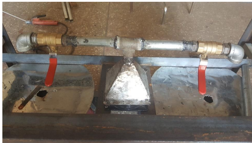
Figure 4.11: Air valve and regulator for controlling air flow to charcoal compartment
