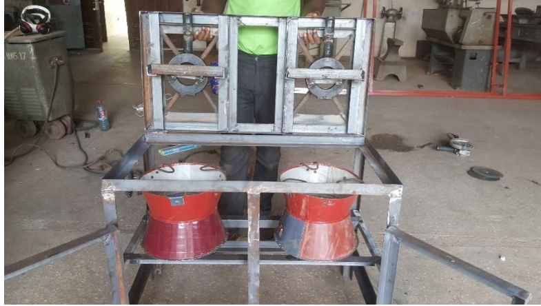
Figure 4.7: The charcoal compartment undergoing fabrication and fixing
