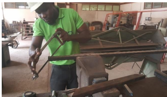
Figure 4.4: Cutting of Main Frame components
