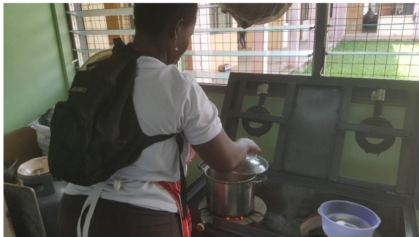
Figure 3.4: IAP meter strapped behind cook for collection of data during the cooking process
