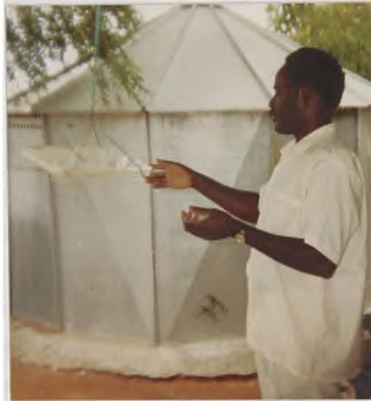
Figure 52. Field improvisation of a rocker during incubations. Note the suspended tray.
