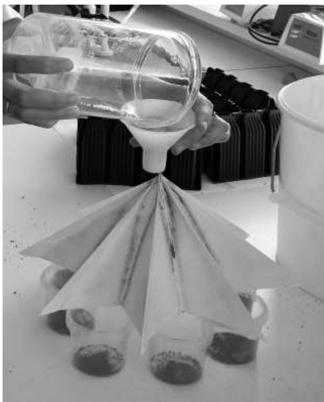
Figure 18. A paper cone riffle splitter used in generating subsamples. Each sample splitting produces 8 subsamples (splits).
