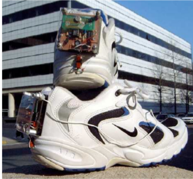
Figure 1.3: A shoe-mounted piezoelectric energy harvesting by [9].
