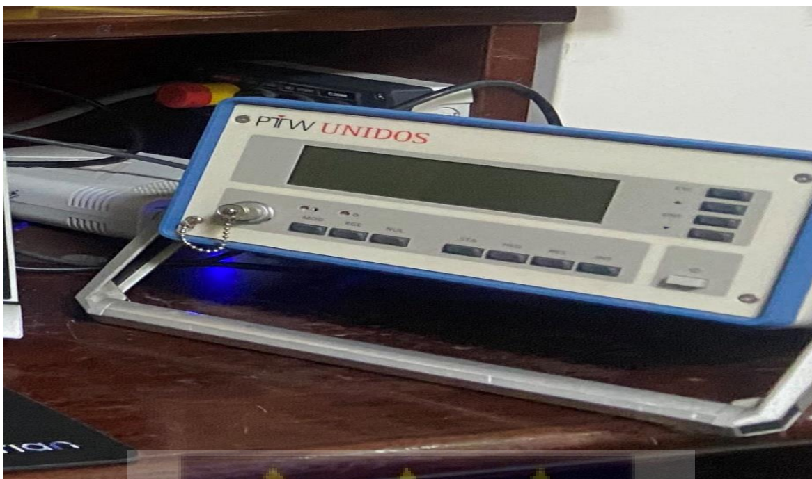
Figure 3.7 PTW Unidos Electrometer (Field work, 2024)
