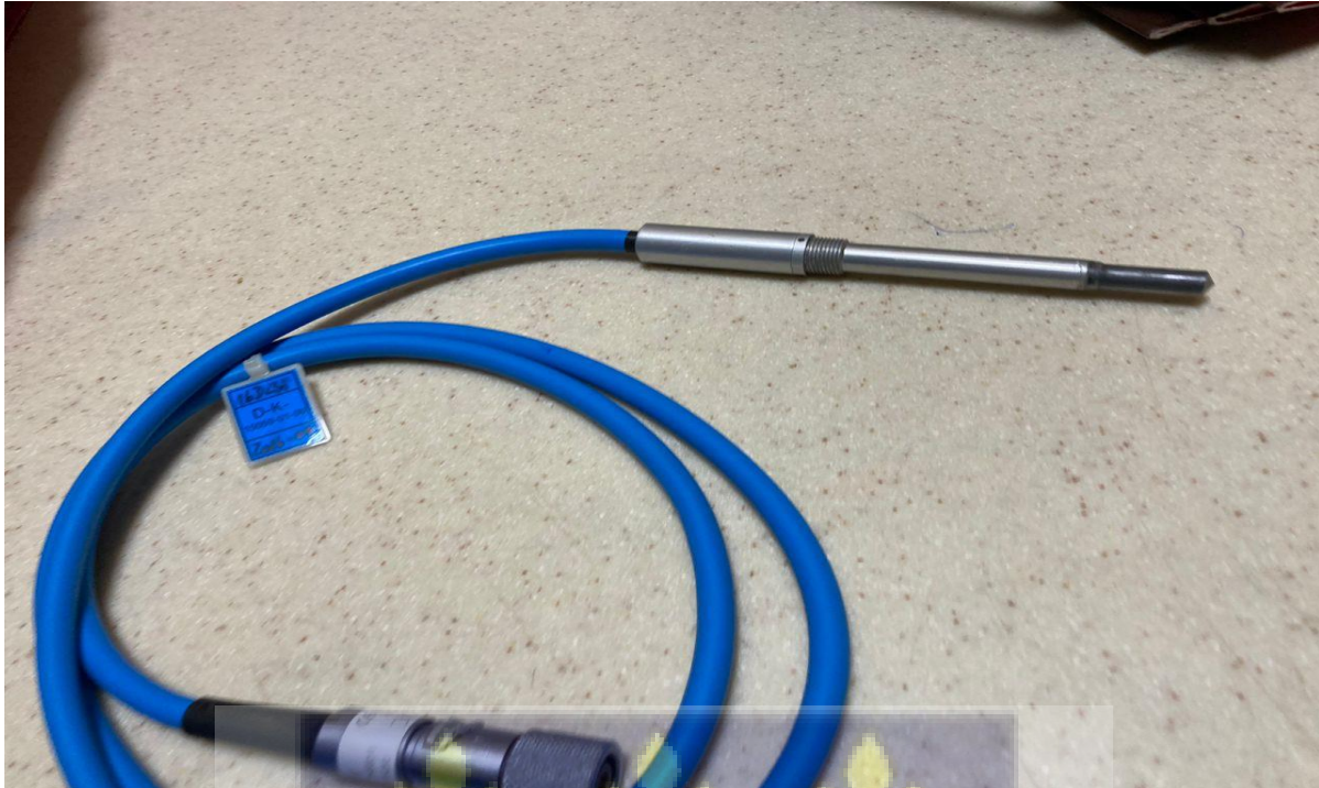
Figure 3.4: PTW 30013 Waterproof Farmer ionization chamber (Field work, 2024)
