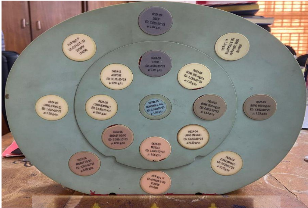
Figure 3.3: Electron Density Phantom model 062M (Field work, 2024)
