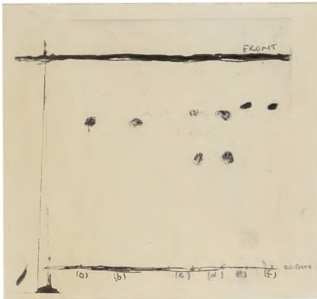
FIGURE 5b CHEMICAL CONFIRMATORY TESTS FOR THE PRESENCE OF AFLATOXIN B 1 IN KOKONTE SAMPLE EXTRACTS.
