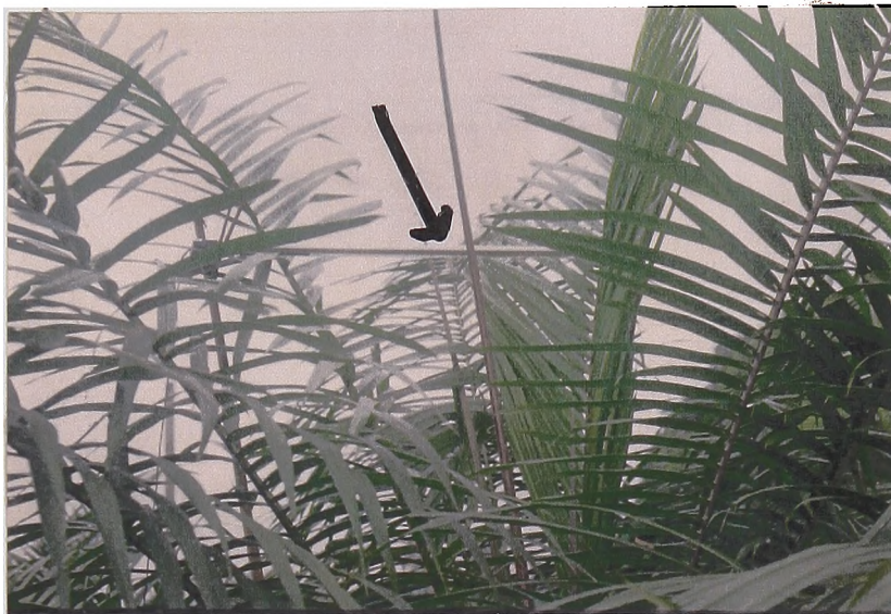
Plate 3.5 Tube Solarimeter installed above the Canopy of oil palm (arrowed)
