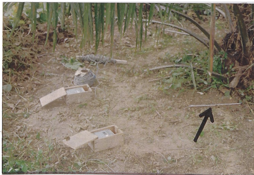
Plate 3.6 Tube Solarimeter installed beneath the canopy of the oil palm (arrowed)
