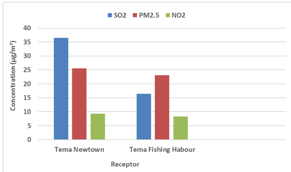
Figure 4.10: Predicted Daily Average Concentrations of SO 2 , NO 2 and PM 2.5 at south eastern receptors in the Study area
