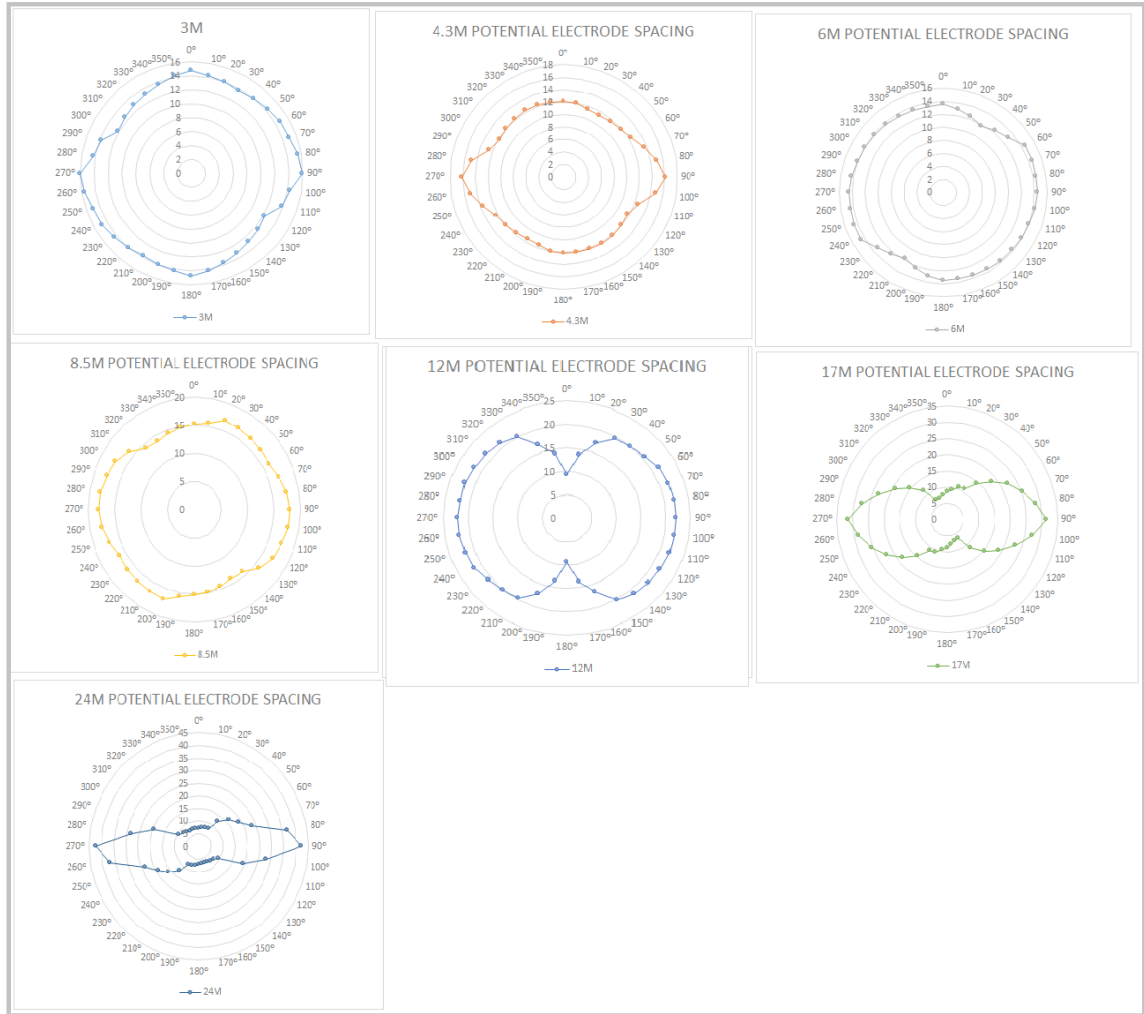
Figure 70: Wenner Azimuthal array plots for KP4
