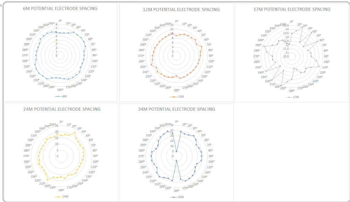
Figure 71: Wenner Azimuthal array plots for KP9
