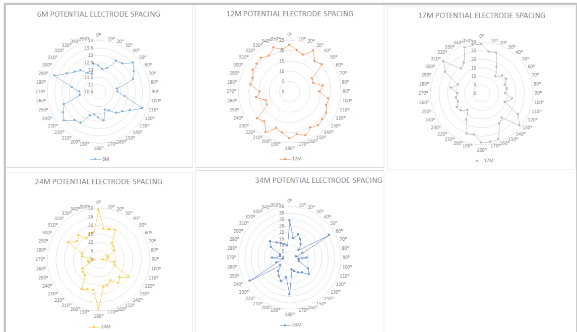
Figure 72: Wenner Azimuthal array plots for KP10
