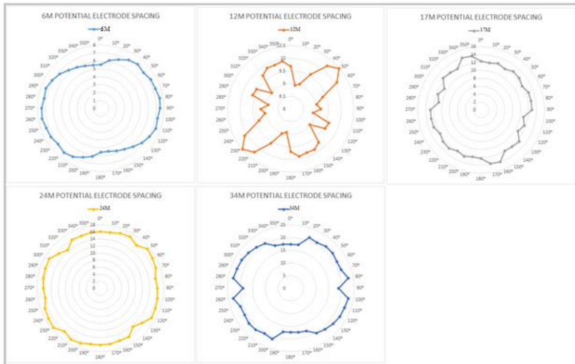
Figure 55: Plots of Wenner Azimuthal resistivity sounding at survey point KP7
