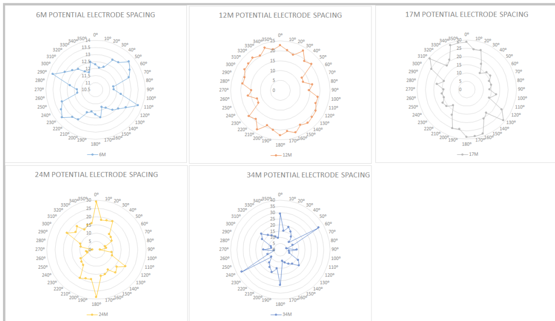
Figure 75: Wenner Azimuthal array plots for KP14
