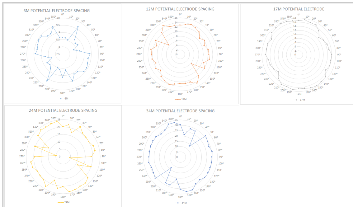
Figure 74: Wenner Azimuthal array plots for KP13
