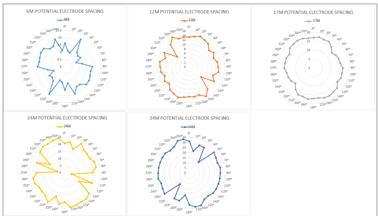
Figure 56: Plots of Wenner Azimuthal resistivity sounding at survey point KP8
