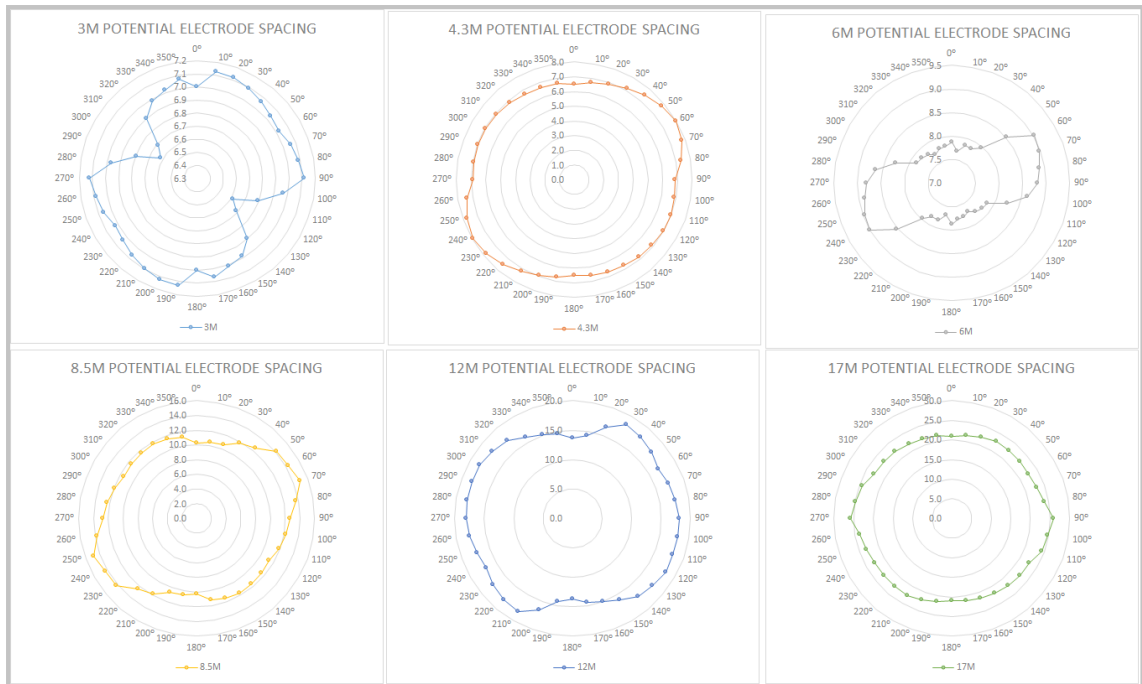
Figure 68: Wenner Azimuthal array plots for KP1
