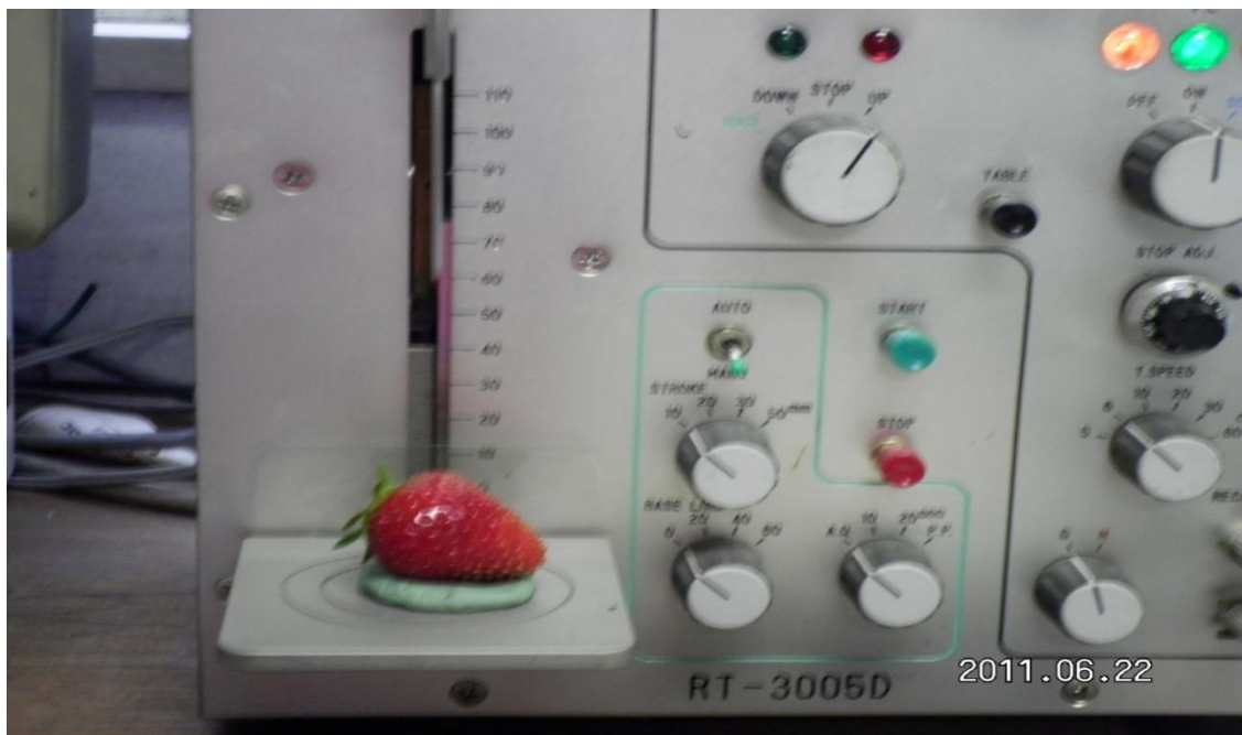
Figure 4: Penetrometer (Fudoh Rheometer RT-3005D) used for measuring fruit firmness during the study
