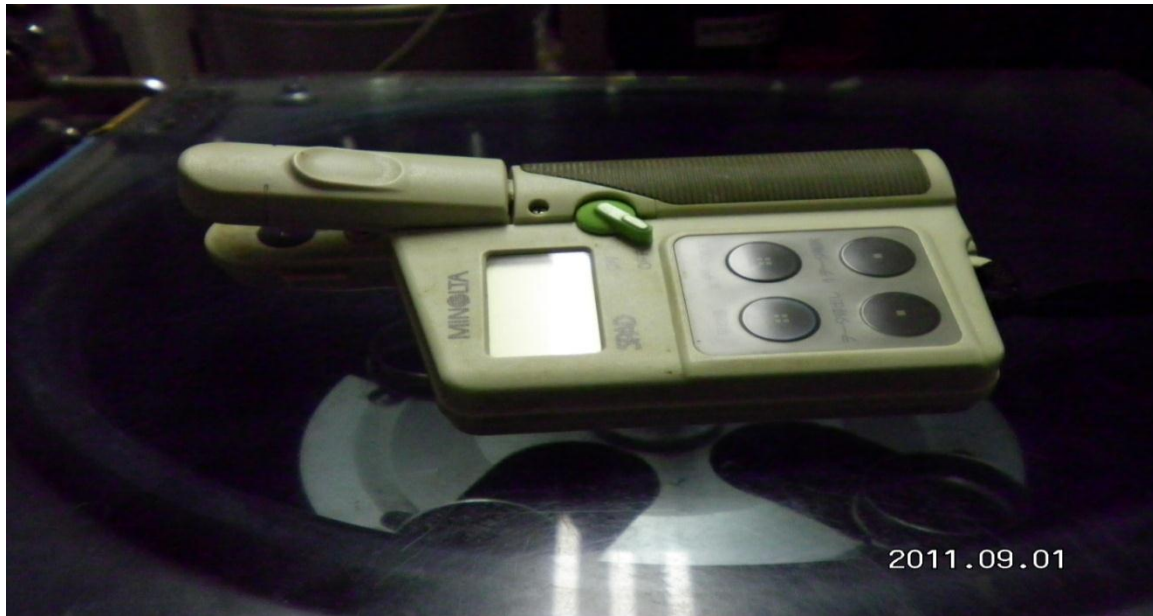
Figure 3: Chlorophyll meter (Model SPAD-502, Minolta, Japan) used for measuring leaf chlorophyll during the experimental period
