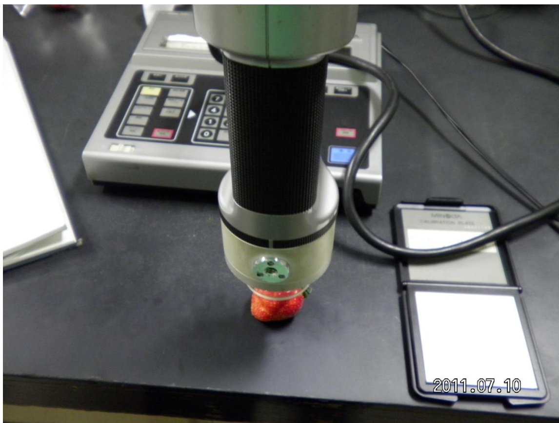
Figure 5: Colorimeter (Minolta, Model CR-300, Osaka, Japan) used for measuring fruit colour during the study
