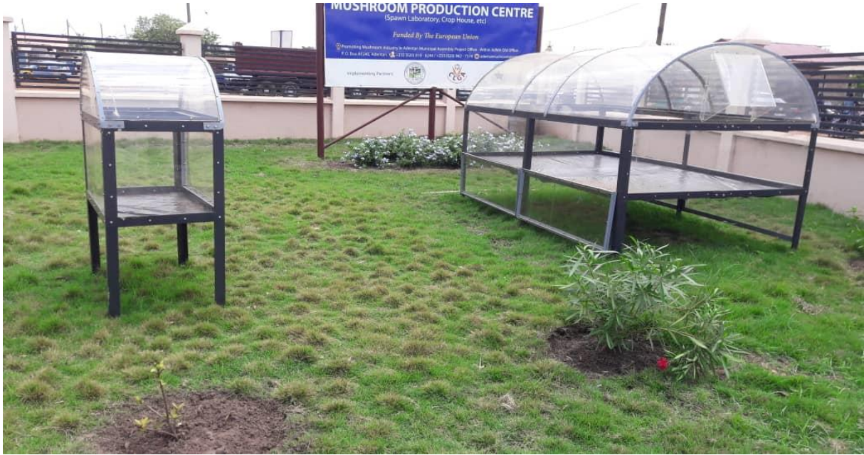
Picture A showing a section of the PROMUSH mushroom training centre with solar dryers for processing fresh mushrooms
