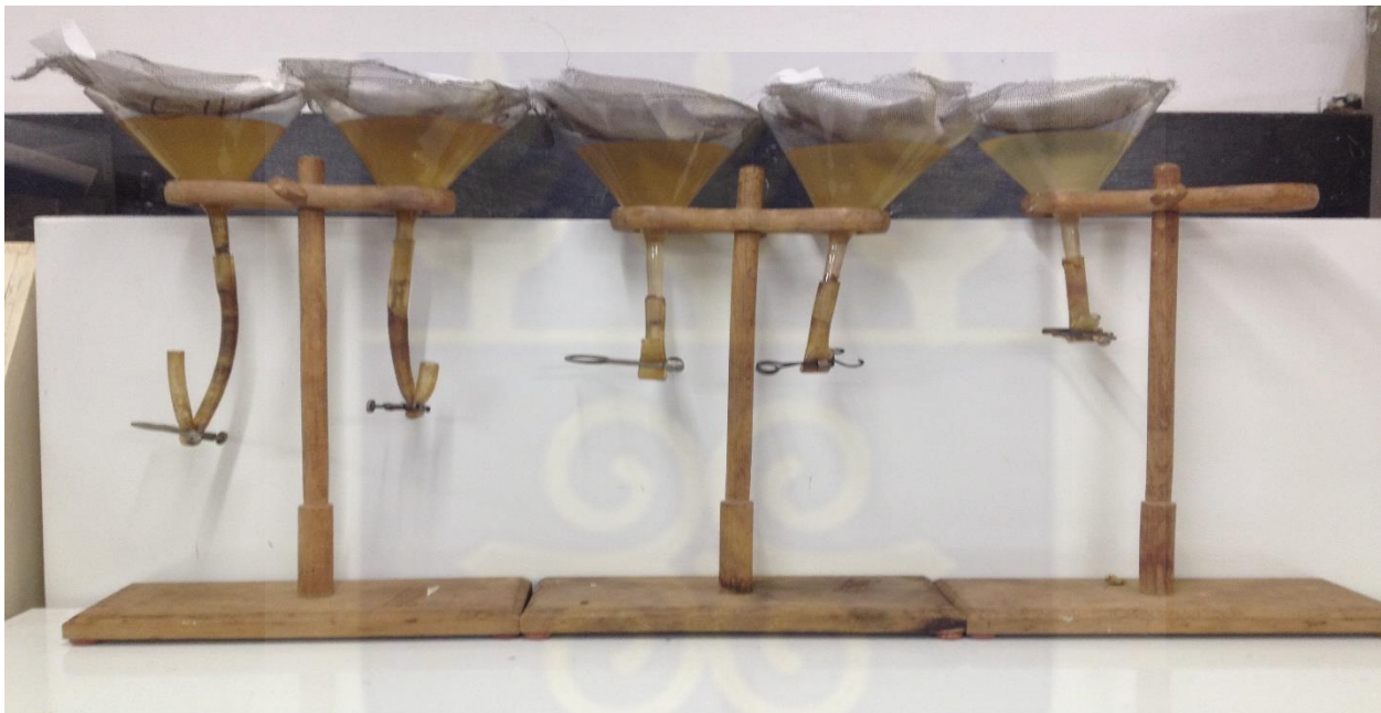
Figure 4. Setup of the Baerman funnel method of extracting nematodes from yam tuber peels
