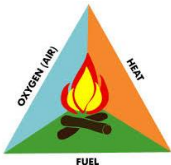
Figure 2.1: The fire triangle Adapted from (Devine, 2015)
