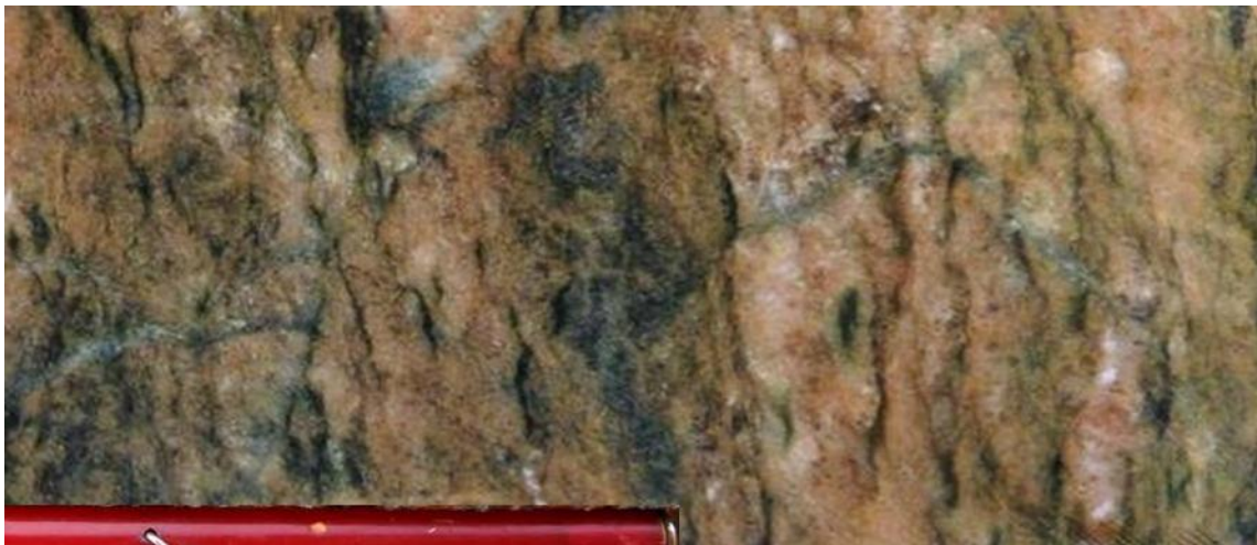
Fig. 2.2 Brittle-ductile shear-breccia zone fabric located west of the mineralized zone at Paboase (low or no Au grade) (Beeson, 2011).
