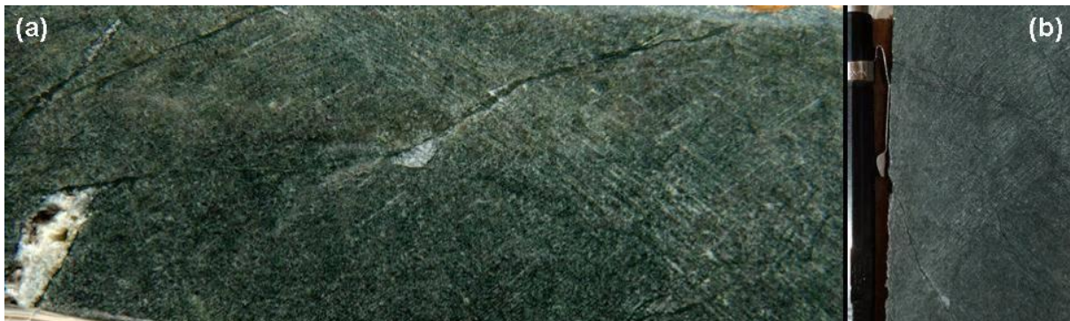
Fig. 2.6 Basalt showing chlorite-carbonate alteration and chloritic fractures (Beeson, 2011).
