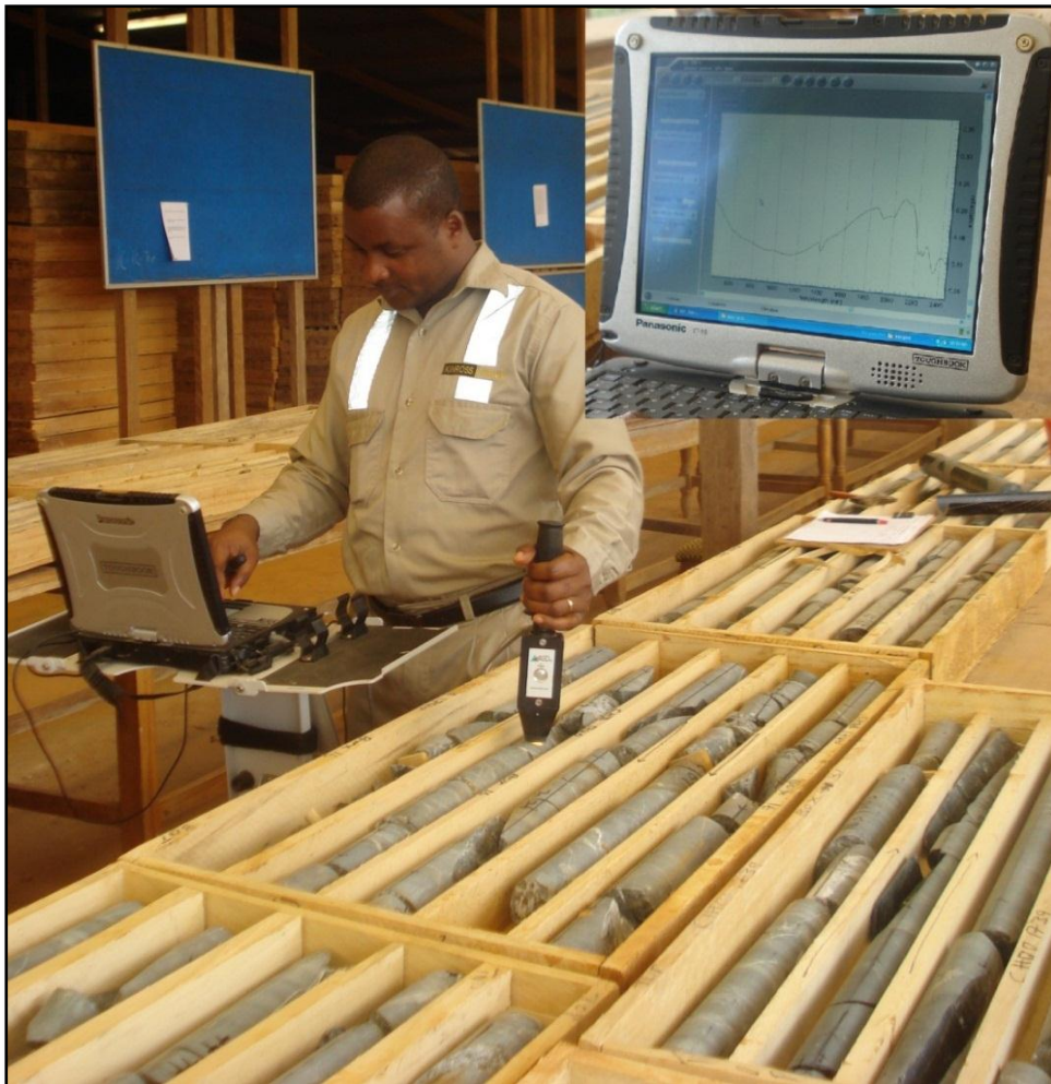
Fig. 3.1 Measuring spectral data using ASD Terraspec Spectrometer.
