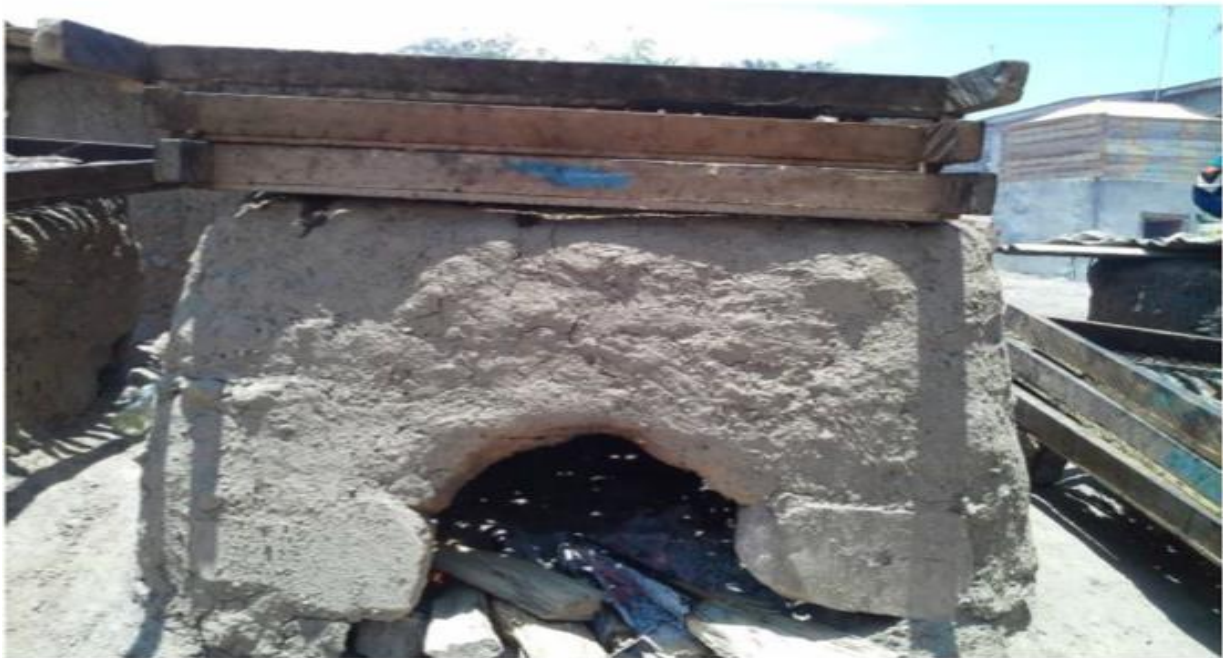
Figure 2.5 “Chorkor” oven with firewood in combustion chamber and mounted fish trays..
