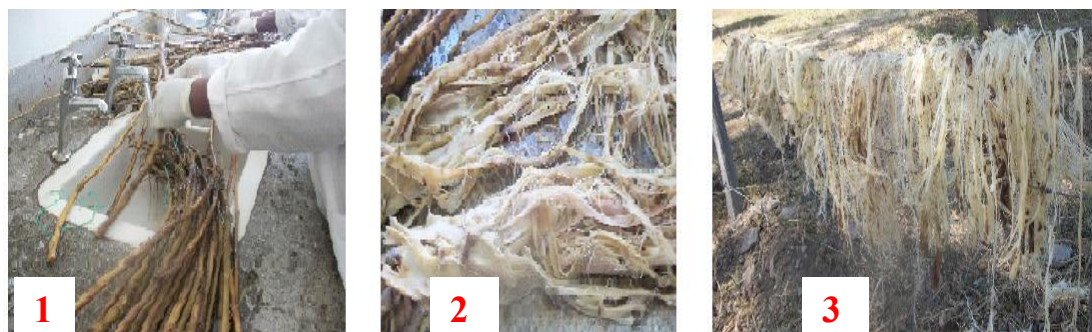
Fig. 2.3b: Extracting bast fibre from roselle; (1) soaking of stems, (2) detached fibres and (3) drying of detached fibres.
