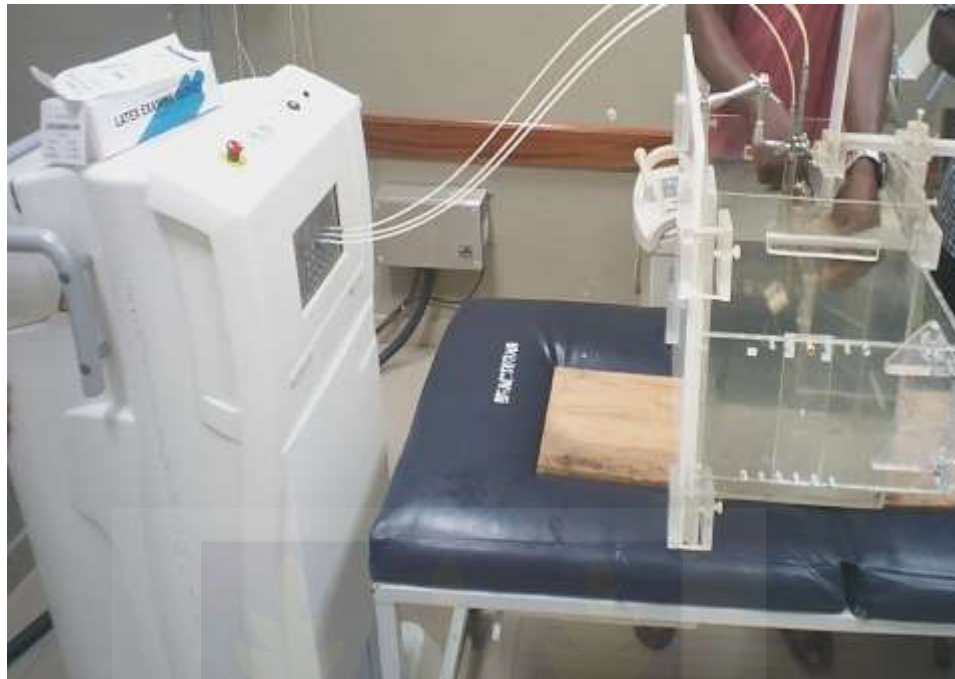
Plate 3.2.2b: Set up showing change of card in holder and putting film in for dose delivery
