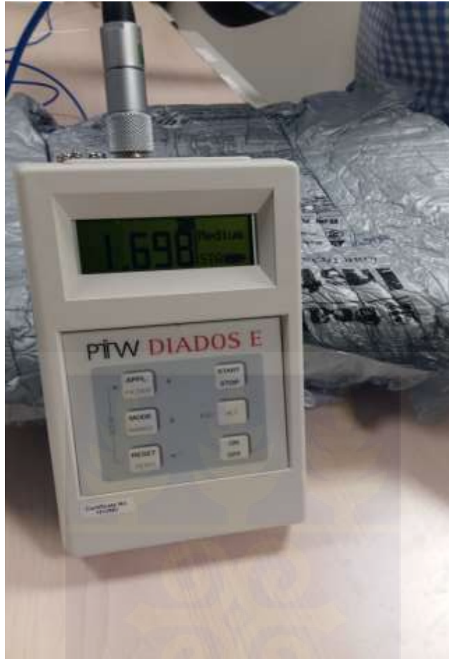
Figure 3.5: Picture of Ion Chamber with integrated Electrometer [Field work 2017]
