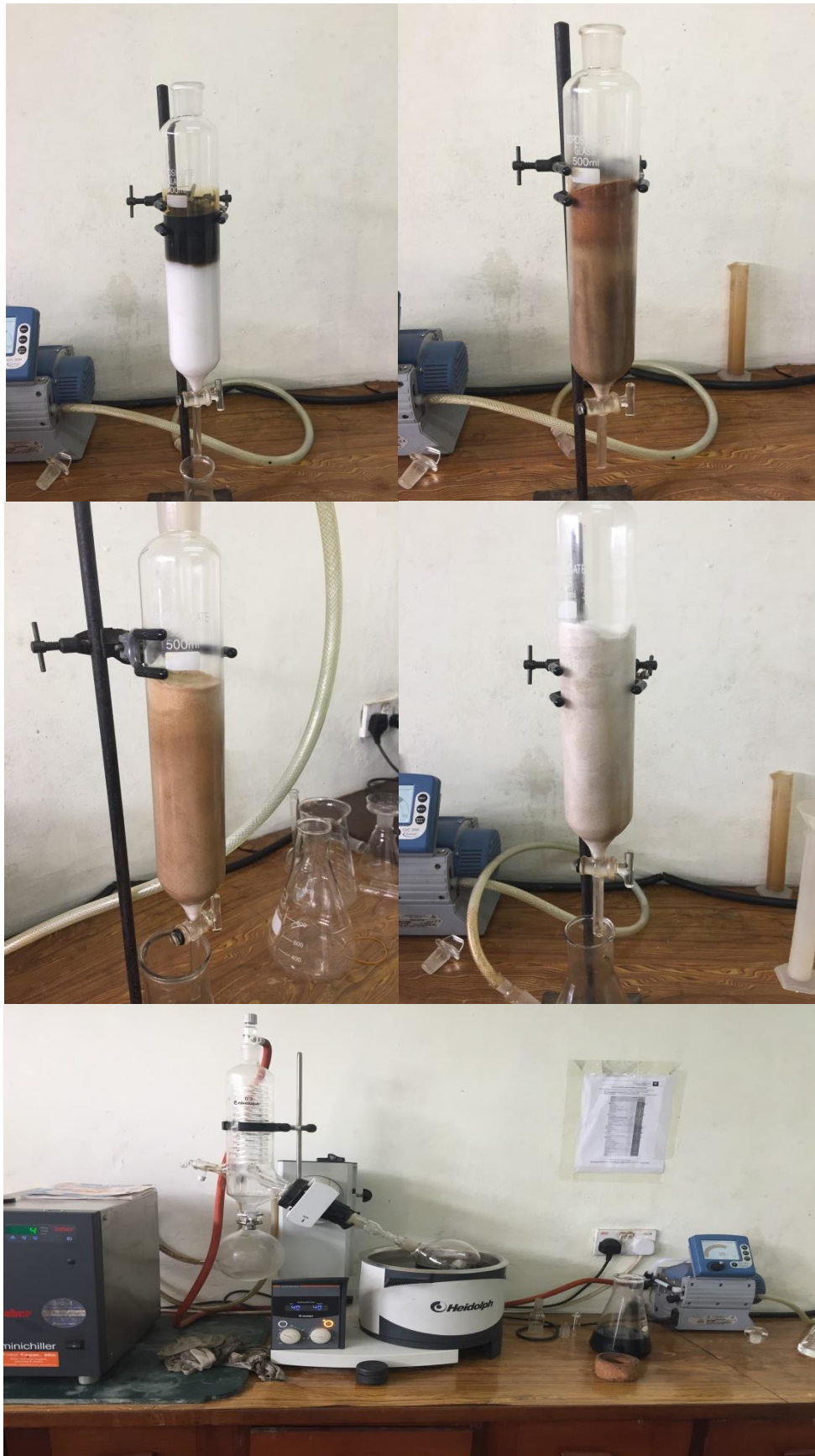
Figure 3. 7 A picture of the setup used in separating the various fractions of the crude oil.
