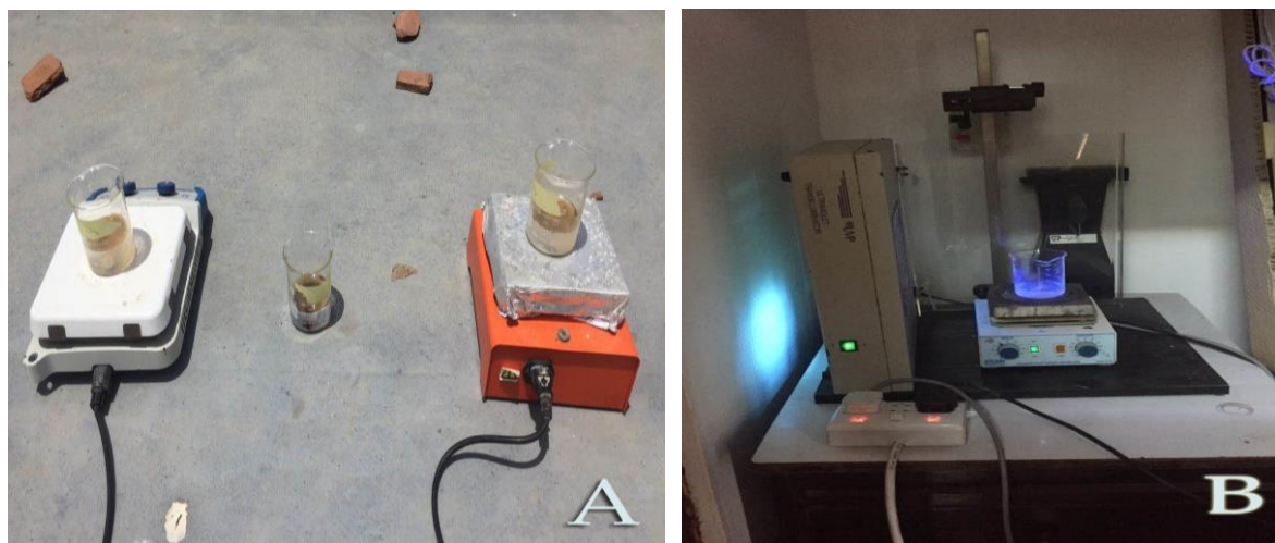
Figure 3. 9 Pictures of the Photodegradation of the crude oil fractions under (A) sunlight and (B) UV irradiation.
