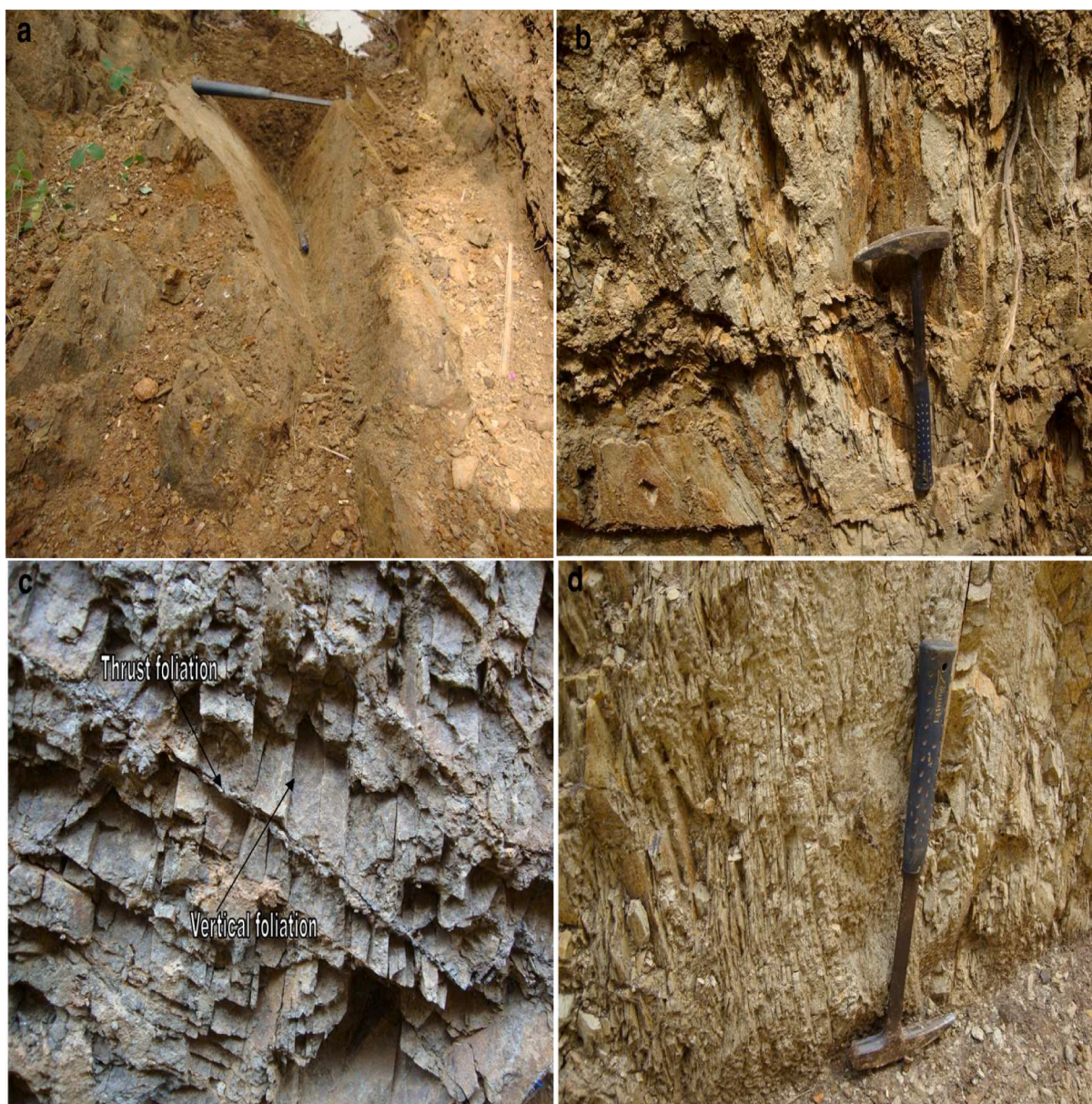
Fig. 14. (a) Fold-like structure due to crossed foliations (b) Sub-vertical foliation in schists (c) Vertical parallel planar foliation (surfaces) cut across by sub-horizontal east dipping thrust foliation (d) Vertical shear foliation in quartz-muscovite schist.
