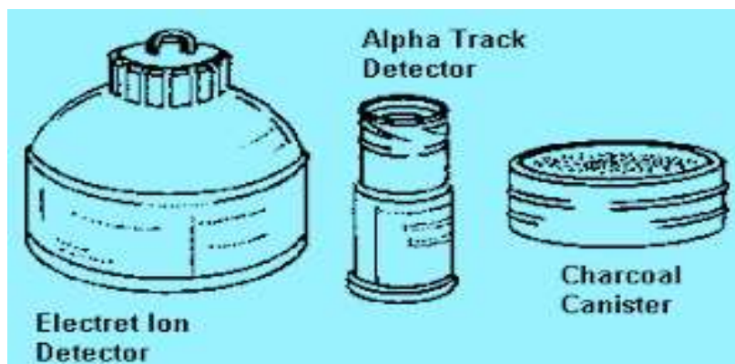
Figure 2.2: Radon gas measurement devices and their characteristics
