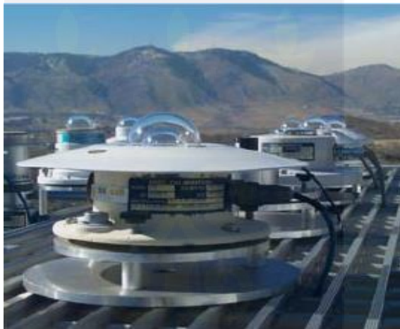
Fig 1.4: Pyranometer for measuring global horizontal radiation. (Adapted from Stoffel and Wilcox, 2004).
