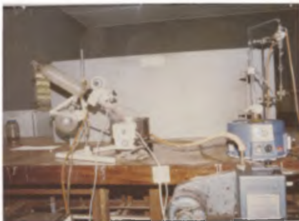
Plate 3. Clavenger apparatus (b) and rotary vacuum evaporator (a) used to extract and concentrate crude oils.
