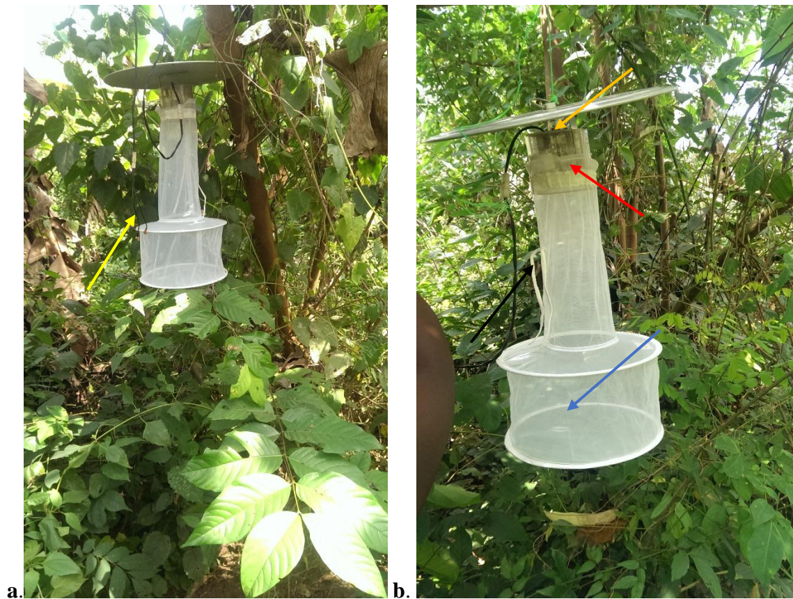
Fig 3.2: Light trap set at different sites on the field. Both images (a&b) display light traps set on the field during the day. Yellow arrow in a. shows where the power source is attached, orange arrow shows position of attraction source (fluorescent bulb), red arrow shows position of fan, blue arrow shows net which contains insects after capture & black arrow shows rope for tying the net to keep insects intact.
