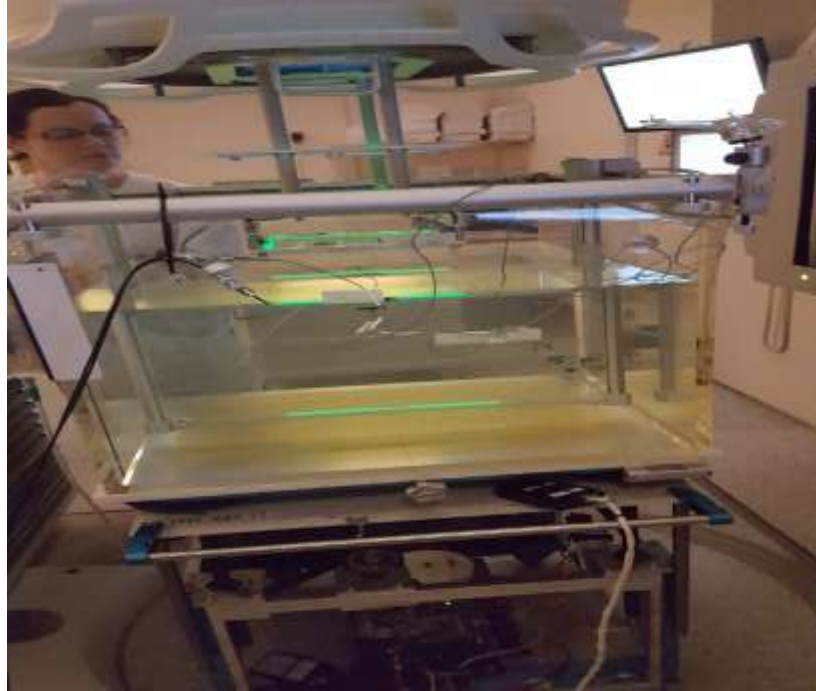
Figure 3. 4: Setup for checking the beam quality and beam profiles of electrons and photons (St. Olav's hospital)
