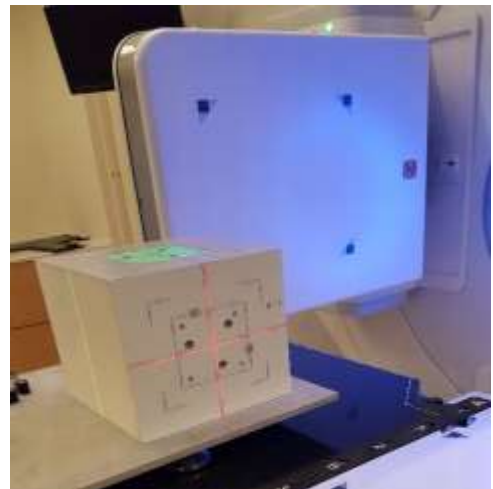
Figure 3. 9 The setup of monthly QA phantom for geometrical checks (St Olav’s hospital)
