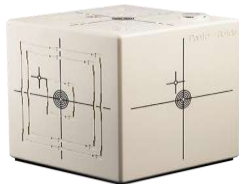
Figure 3. 11: A picture of Penta Guide phantom for XVI QC (St Olav’s hospital)
