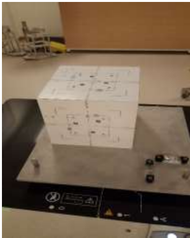
Figure 3. 8: A home built monthly QA Phantom (St Olav’s hospital)
