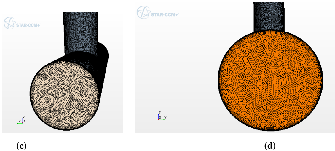
Figure 3.7: Meshed Domain; Mixing-Junction (a), inlet (b) & (c), outlet (d)
