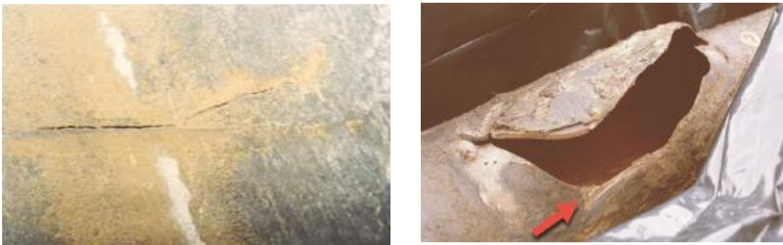
Figure 2.2: Thermal fatigue failures (Jayaraju et. al., 2011)
