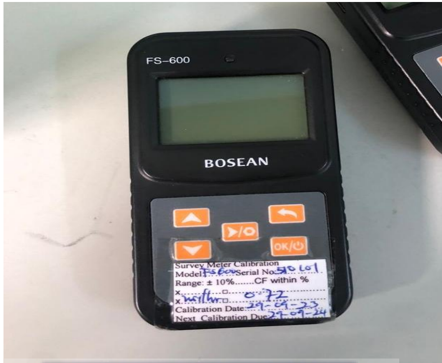
Figure 3.3: A pictorial view of the Bosean survey meter used for cross calibration
