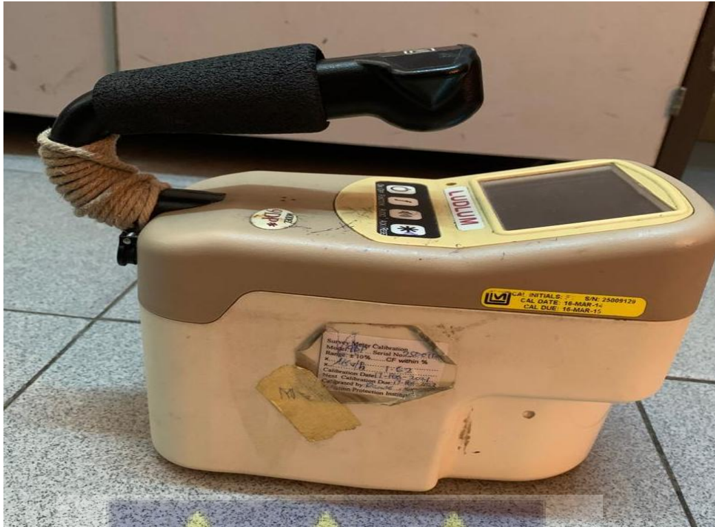
Figure 3.2: A pictorial view of the Ludlum survey meter
