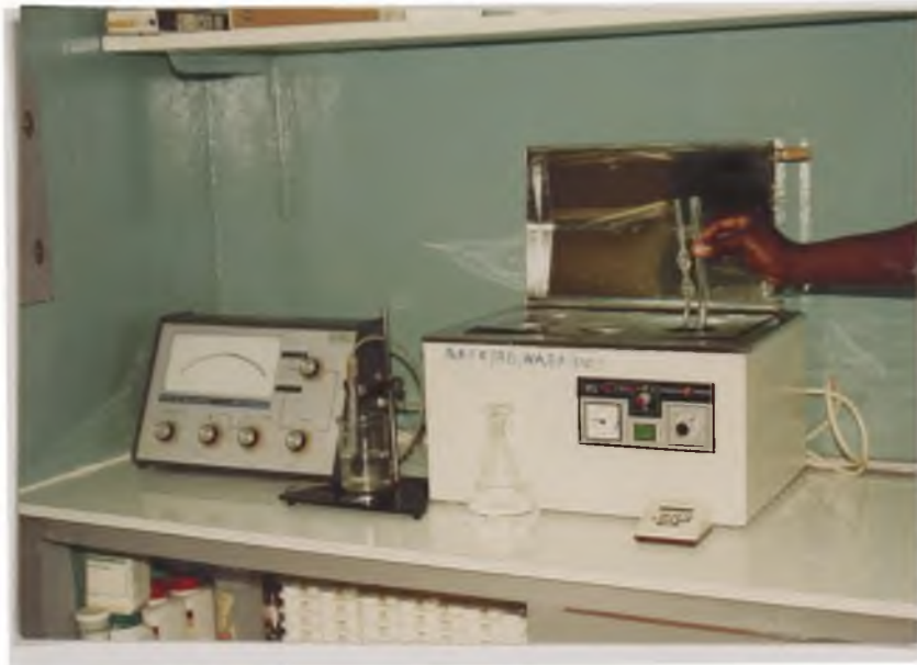
Plate 1. Photograph of set up used in determining changes in viscosity of different media caused by amylase, pectinase and cellulase enzymes produced by T. viride , R. oryzae , A. niger and L.plantarum . ( Note the hand holding the Fenske-Ostwald Viscometer)
