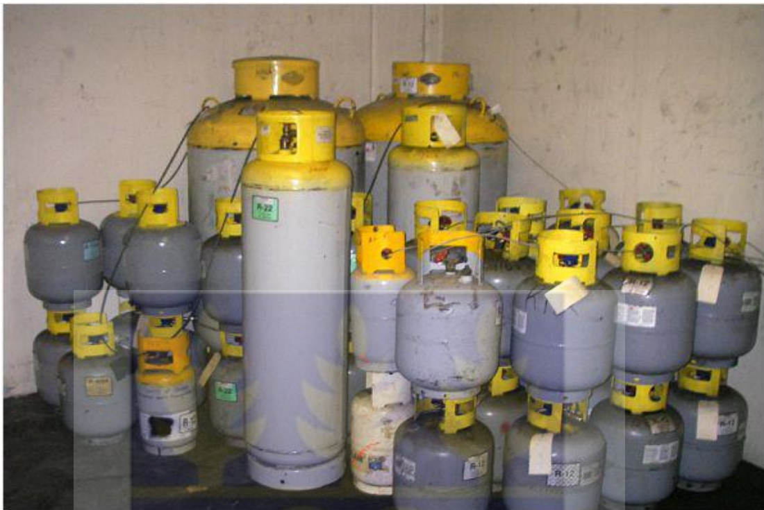
Figure 4.10: Recovered CFC-12 in cylinders awaiting export at the EPA ODS lab.
