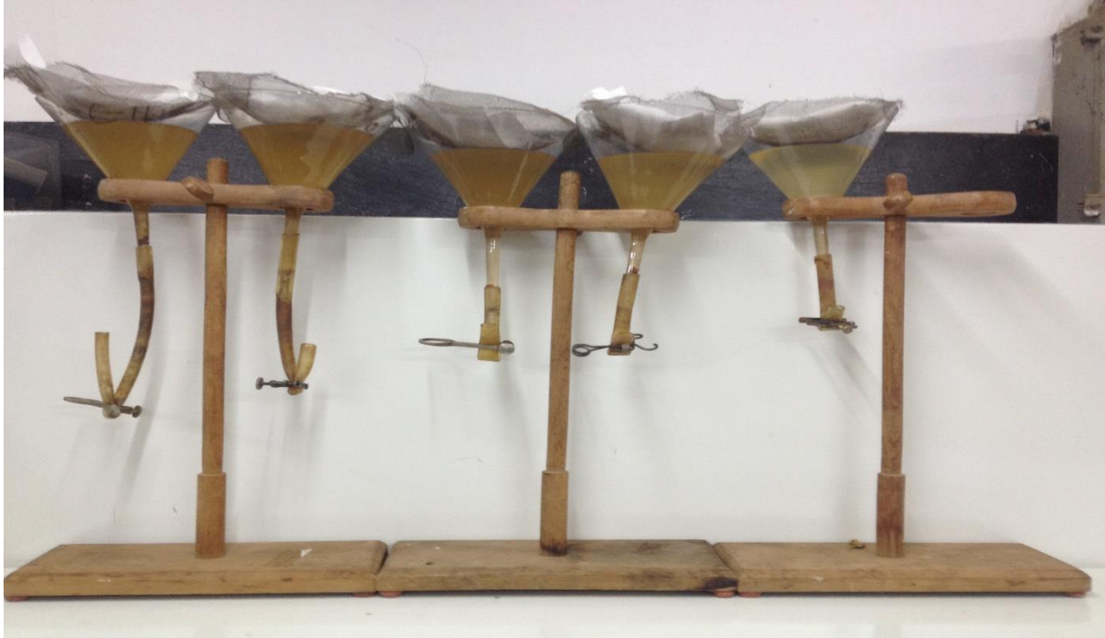
Fig. 2: Set-up of Baermann funnel method used for nematode extraction from tomato roots
