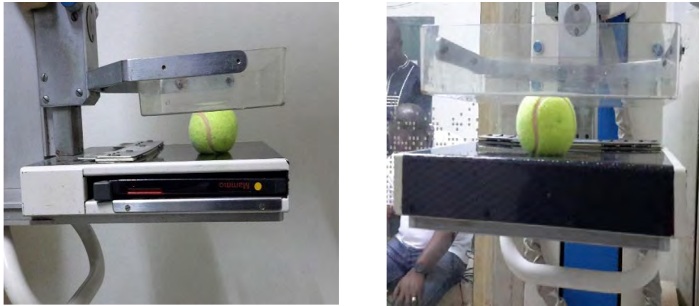
Figure 3.9: Setup of compression paddle alignment test
