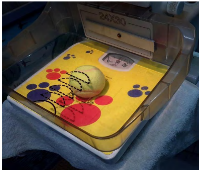
Figure 3.10: Setup of compression force test
