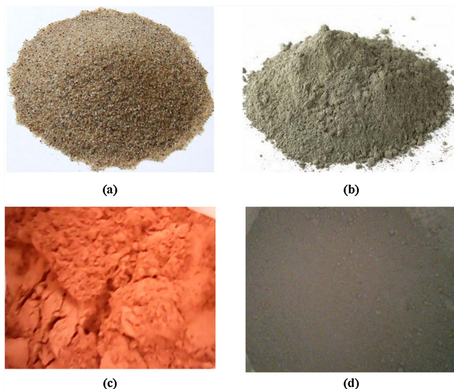
Fig. 3. Materials used; (a) river sand as fine aggregates; (b) ordinary Portland cement (Diamond, class 42.5N); (c) Bauxite red mud and (d) red mud cement composite.
