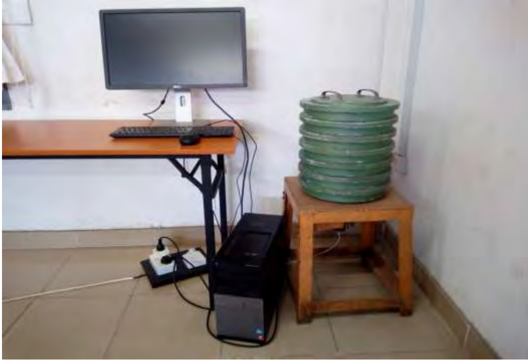
Figure 3.3: Gamma spectrometry system with NaI detector
