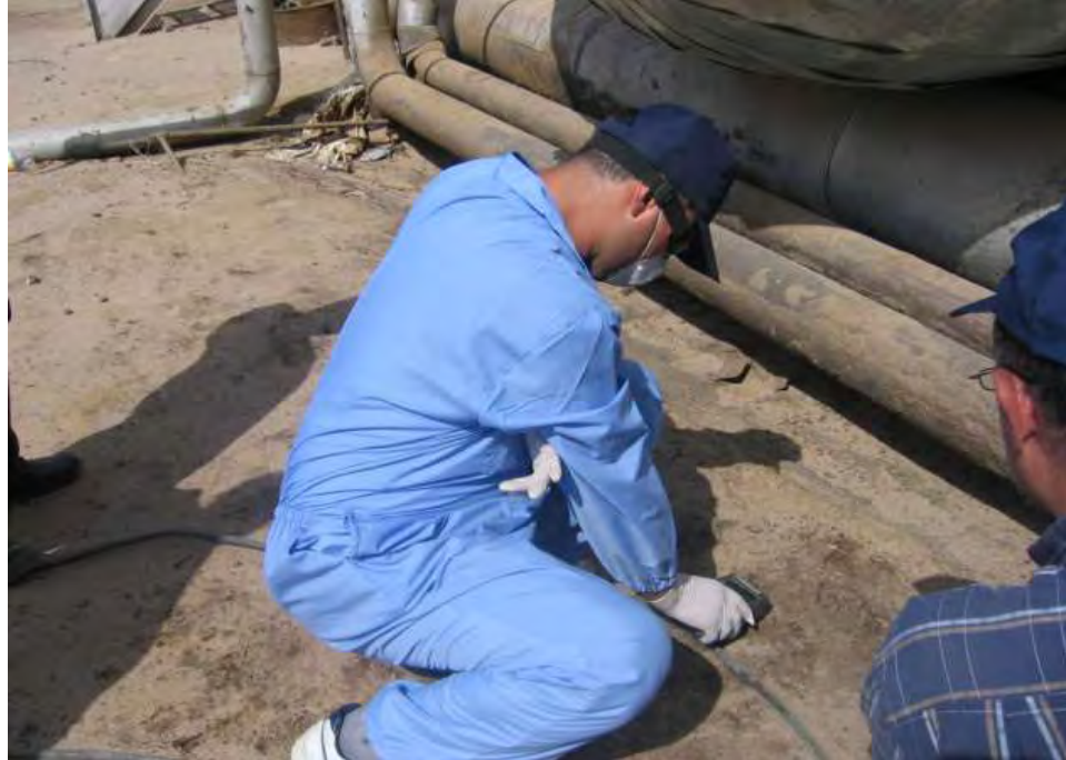
Plate 2.1: Monitoring the outside of equipment/plant with a dose rate meter (Zaidan, 2010)
