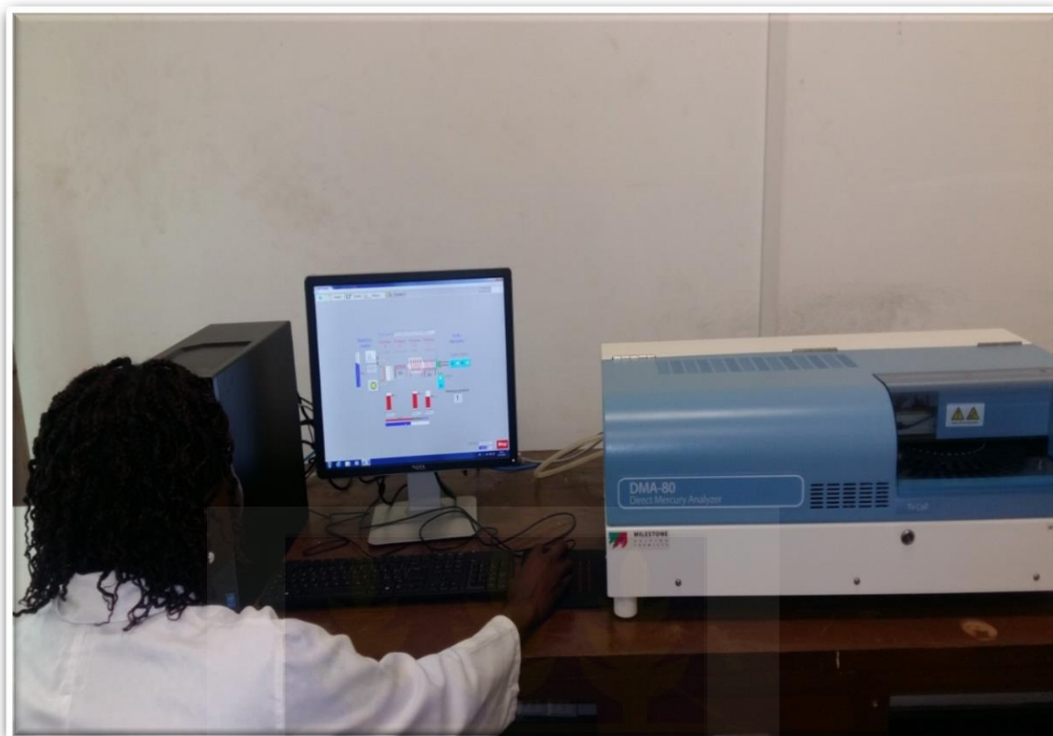
Figure 3.1: Direct mercury analyser connected to a desktop computer (Image taken with Samsung Camera ST76 x 1Mag.)
