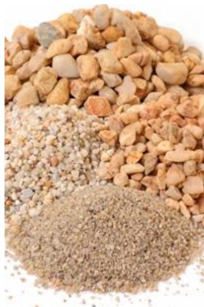
Figure 3-6. Typical grades of sand and gravel for filter bed (Source: Neumann Group, 2010)
