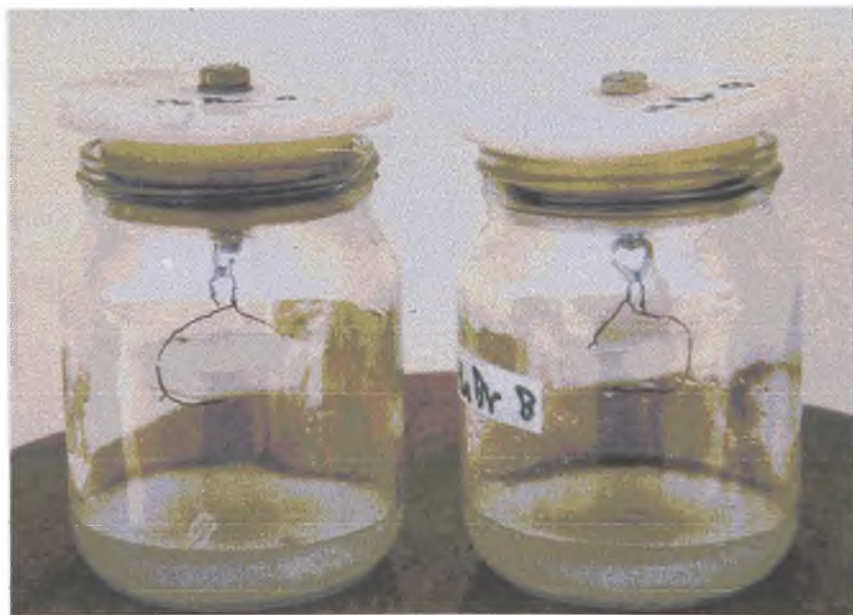
Fig 3.4: Containers used for sorption isotherm experiment
