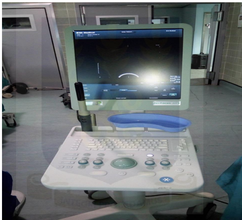
Figure 3.2. A pictorial view of ultrasound unit and rectal probe used at the theatre for the procedure
