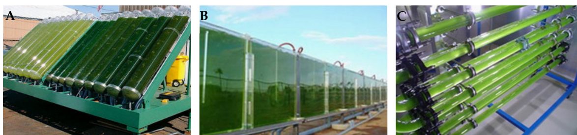
Figure 3. Photobioreactors for algae cultivation: (A) inclined tubular photobioreactor, (B) flat-plate photobioreactor, and (C) horizontal/continuous photobioreactor [82].
