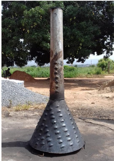
Plate 1 Locally manufactured kuntan kiln
