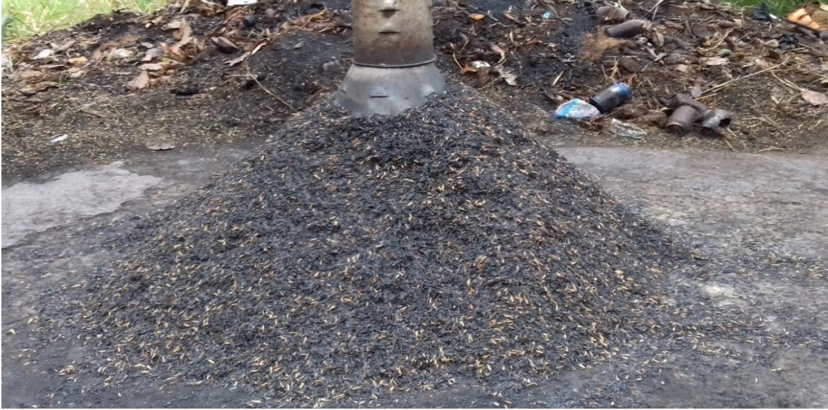
Plate 3 Partially charred rice husk biochar
