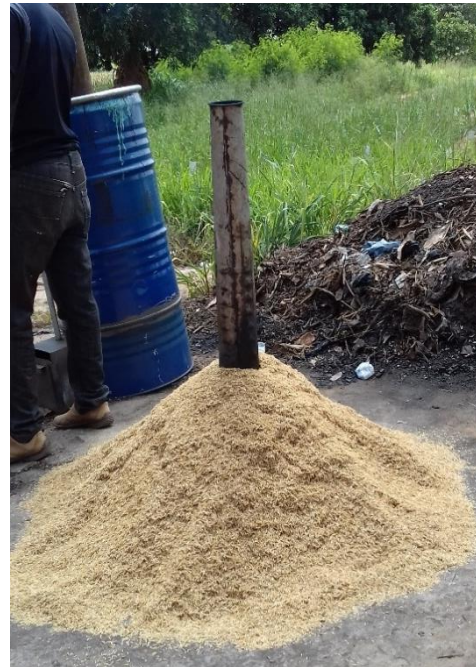
Plate 2 Rice husk feedstock under charring
