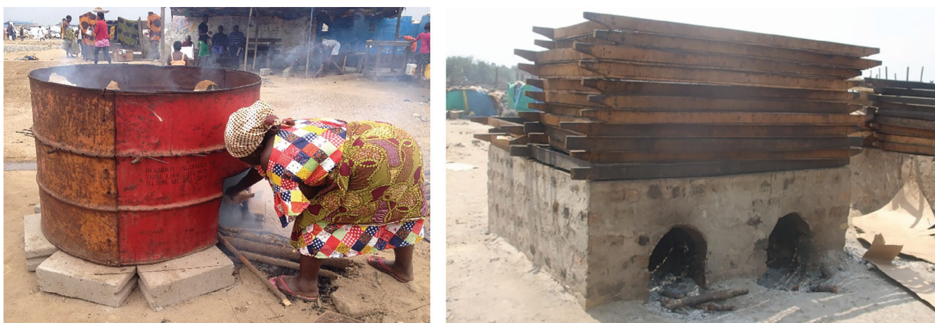
Figure 1. Traditional kilns for fish smoking in Ghana. Metal drum kiln (left) and Chorkor smoker (right).
