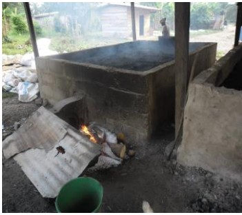
Roasting of palm nuts in a locally constructed oven
