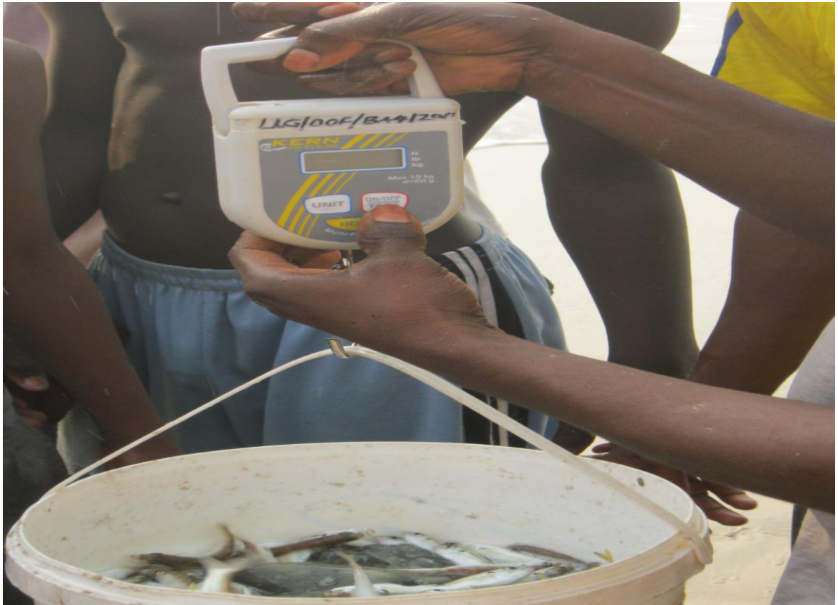
Plate 1: Weighing of fish on the field using field hand scale KERN CH15K20
