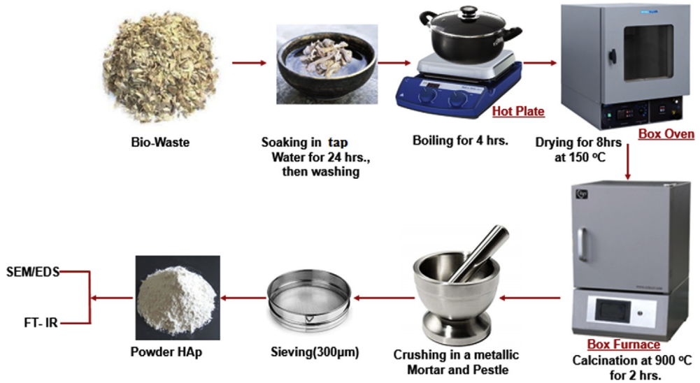
Fig. 4. Schematic of hydroxyapatite preparation and characterization techniques.
