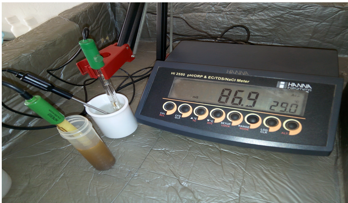
Fig. 3.8 setup for conductivity measurement of the sample's solution
