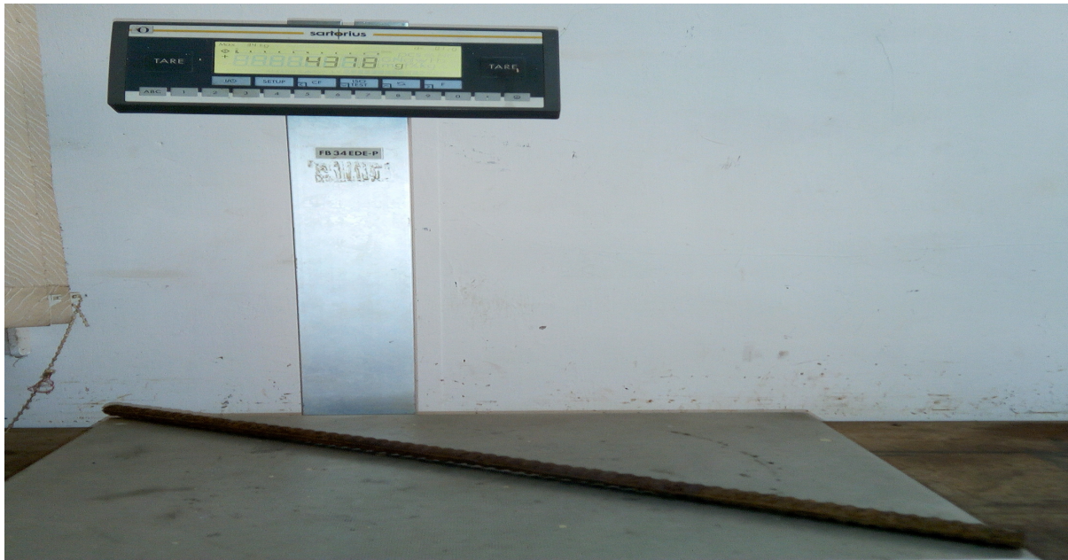
Fig. 3.9 weighing sample before its mechanical test
