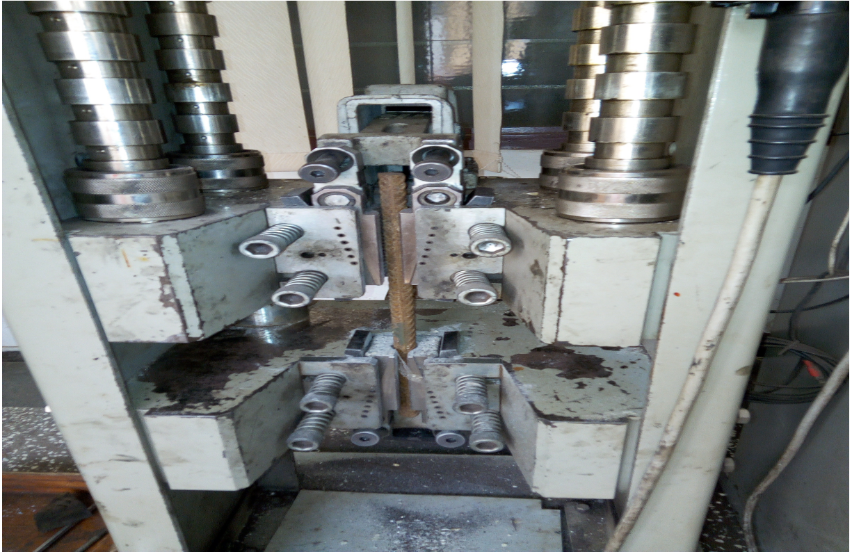
Fig. 3.7 sample being held in good position to start mechanic strength test
