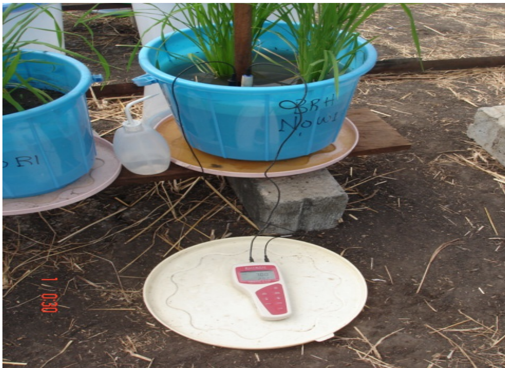
Plate 3. 4 Measurement of soil and floodwater temperature using pH/°C/mV meter.
