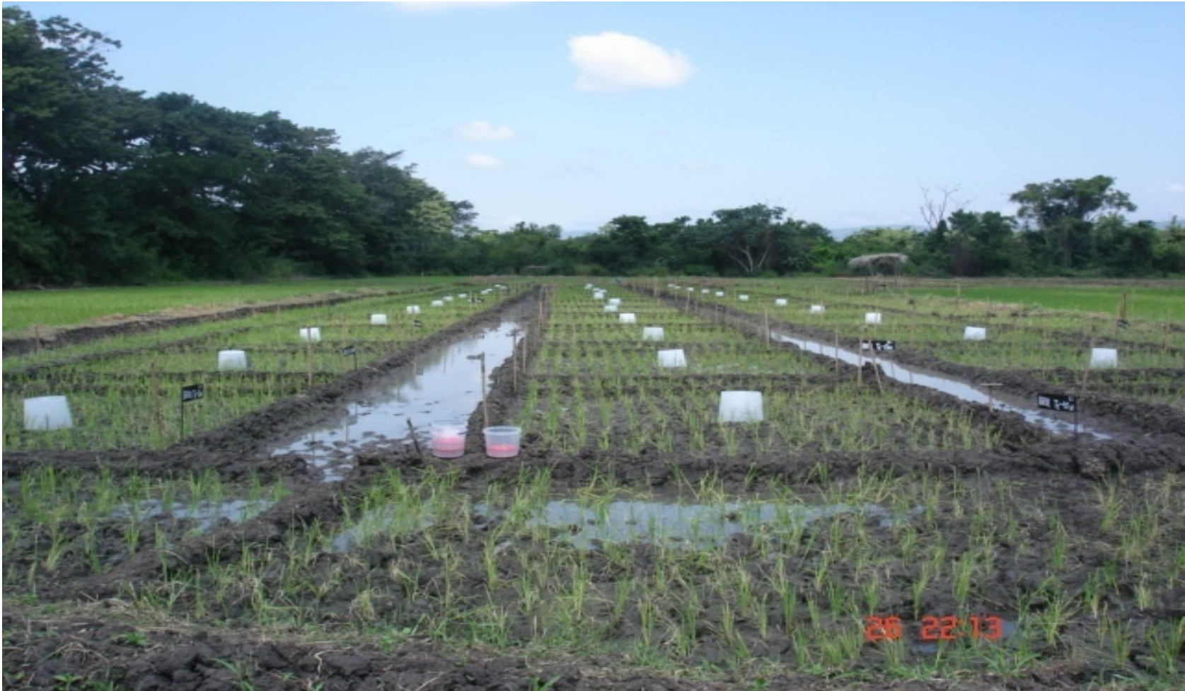
Plate 3. 2 Layout of field experiment showing chambers for trapping effluxed CO 2 .
