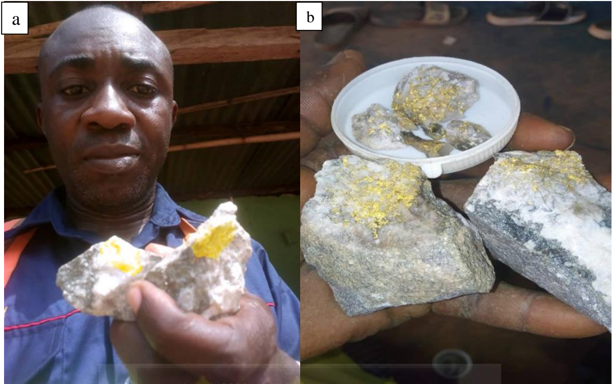
Figure 4.33: a) Auriferous quartz-carbonate rock b) Stockworks hosted by the quartz-feldspar porphyry as observed Cobra Creek and Agyapoma satellite lode gold deposit.
