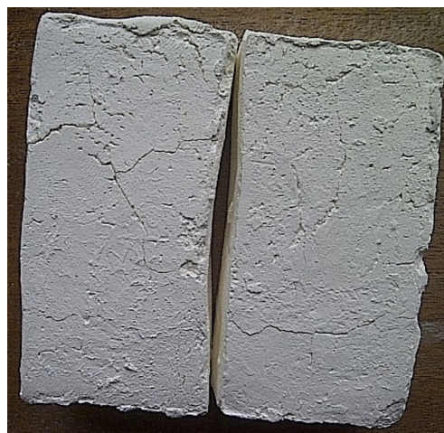
Fig. 16. Porous ceramic with HDPE as pore former showing micro cracks.
